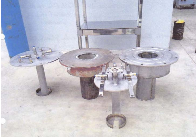
Figure 3. Bomb reactors built in Burma for uranium metal production. The one on the left is discolored from heating. The one on the right has an improved sealing mechanism.
